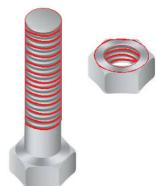
20% loss in converted load through not lubricating the threads.
